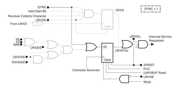
Figure 14–12. Receive Interrupt State Diagram
